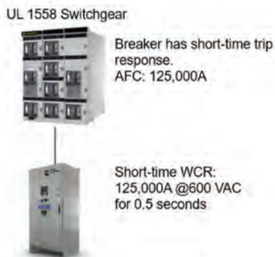
Figure-07 UL1558 Switchgear With UL1066 Breakers Feeding Transfer Switches
